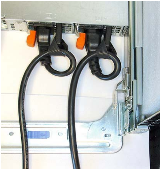
Figure 3: Routing Power Cables Through the Strain Reliefs
